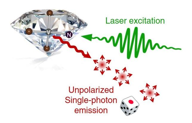
Schematic picture of unpolarized single-photon generation using a compound defect, a nitrogen vacancy center (NV center), in a diamond. Spheres, designated N and V respectively, indicate a nitrogen atom and a vacancy which comprises an NV center in the diamond lattice. Dynamically and statically unpolarized single-photon emission is induced by laser excitation for a [111]-oriented NV center in (111) diamond. Credit: Naofumi Abe
