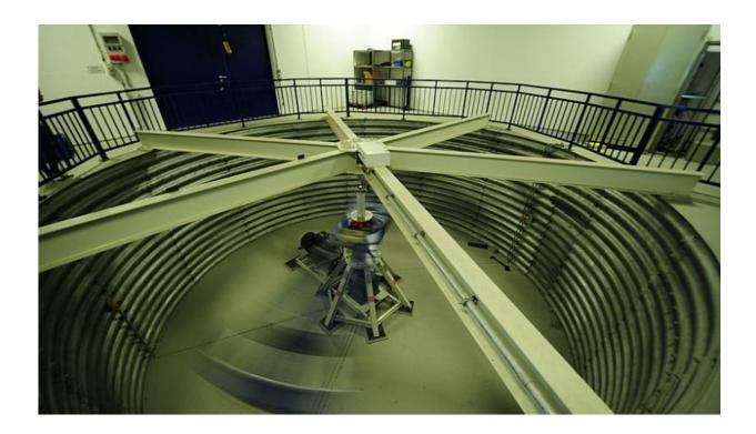
The rotating centrifuge in which the entangled photon source was accelerated to 30 times its weight. Credit: IQOQI/ÖAW
