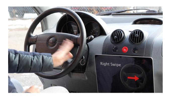
Researchers at Carnegie Mellon University's Human-Computer Interaction Institute have developed a low-cost method of turning a wide variety of surfaces into touchpads, such as this steering wheel Credit: Future Interfaces Group
