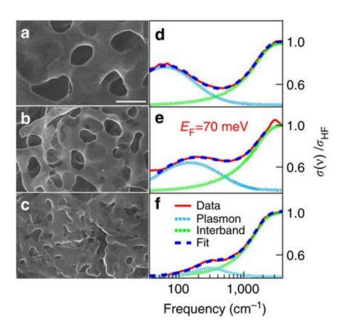
SEM-images of 3-D graphene with different pore size (a,b,c, scale =  $1\mu$ m). Optical properties (d,e,f) change with pore size. Credit: *Nature Communications*: 10.1038/ncomms14885
