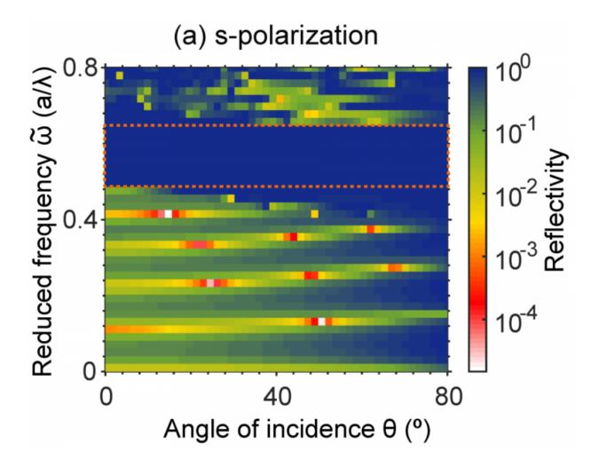
Figure 2: The calculated reflectivity spectra for all orientations of the incident light. Light that cannot enter the crystals is reflected, signaling that these colors are completely forbidden to exist inside the crystals, which is the signature of the photonic band gap. The researchers observe that light for a broad range of colors is always reflected for any angle of incidence and for both orientations, even for
