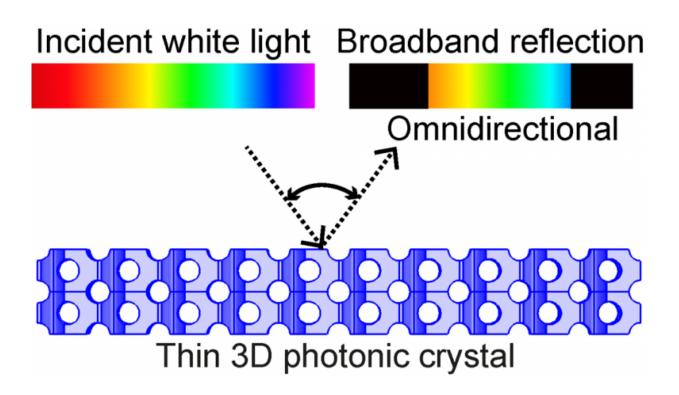
Figure 1: A thin 3D photonic crystal with a diamond-like nanostructure is illuminated by white light from any incident direction (black arrow). Many colors are strongly reflected omnidirectionally irrespective of the incident angle (black arrow). In this example, these are the colors from orange to blue. Credit: University of Twente
