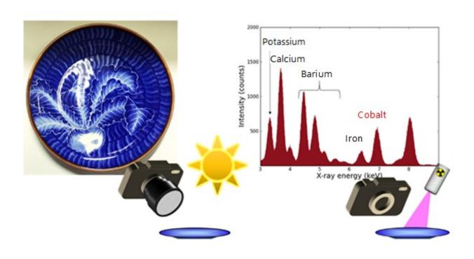
(Left) A ceramic plate used as a measurement sample. Use of a visible light camera allows one to record target objects' shapes and colors as images (The camera used in this study takes black and white images). (Right) X-ray spectra obtained using the same camera. Chemical elements can be analyzed based on differences in energy levels, which represent different X-ray colors, distributed across the X-ray wavelength region. Credit: National Institute for Materials Science
