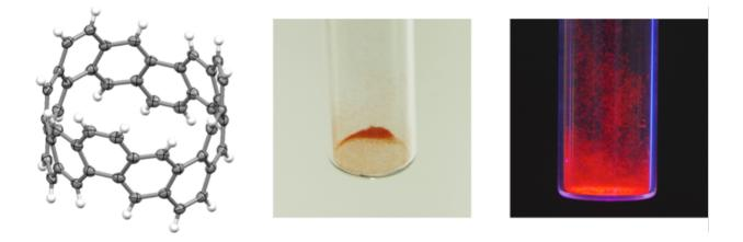
Figure 4. From the left: X-ray structure of carbon nanobelt, crystals of carbon nanobelt under room light, and under UV light. Credit: Nagoya University
