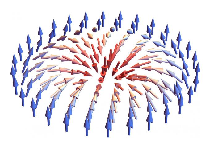
The configuration of spins in a Néel skyrmion. Credit: Zhang et al.
