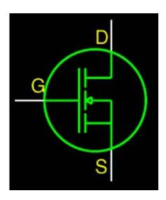
Tensile mechanical stress can have a useful effect for some transistors, where the resulting atomic strain allows its current-carrying electronhole pairs better mobility. However, when that stress is applied to the whole device, as is a popular approach via use of what's called contact etching stop layers (CESLs), the drift region adjacent to the stretched channel is compressed and results in reduced performance.
