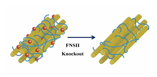
Control (left) and experimental (right) are shown. After flavone synthase II (FNII) is knocked out, rice straw does not produce tricin and its lignin content is reduced by approximately one-third. The glucose yield is increased by 37% after cellulose degradation. Credit: The University of Hong Kong
