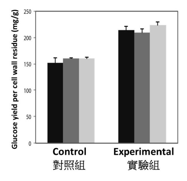
Glucose yield from FNSII-knockout rice straw (experimental) after cellulose degradation is increased by 37%, making it more efficient for ethanol production. Data were collected from three plants in each of the control and experimental groups. Credit: The University of Hong Kong
