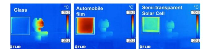
Thermal images are taken by an infrared camera to compare the heat rejection performance of automobile window film, semi-transparent solar cell and glass. Credit: Korea Advanced Institute of Science and Technology (KAIST
