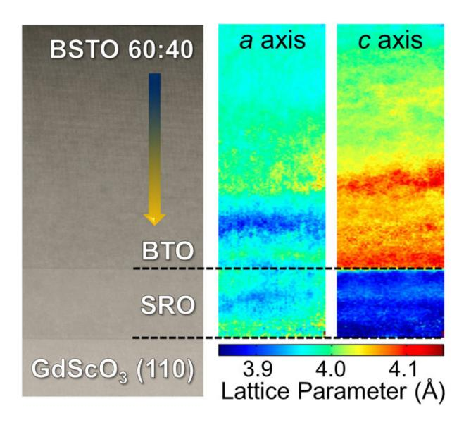
On the left is a low-resolution scanning transmission electron microscopy (STEM) image of a ferroelectric material that is continuously graded from
