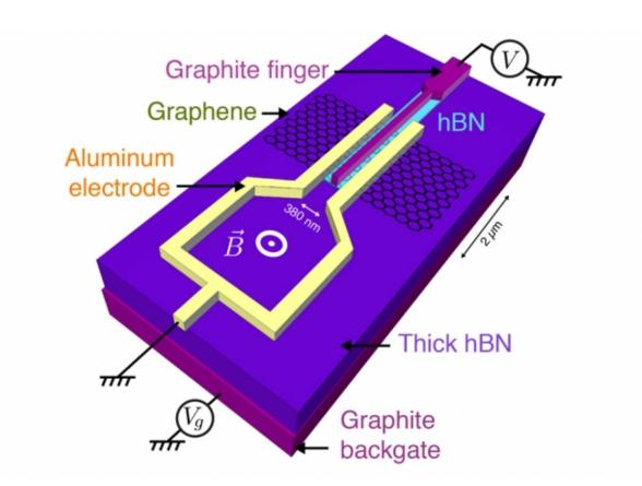
MIT physicists have found that a flake of graphene, when brought in close proximity with two superconducting materials, can inherit some of those materials' superconducting qualities. As graphene is sandwiched between superconductors, its electronic state changes dramatically, even at its center. Pictured is the experimental concept and device schematic. Credit: Massachusetts Institute of Technology
