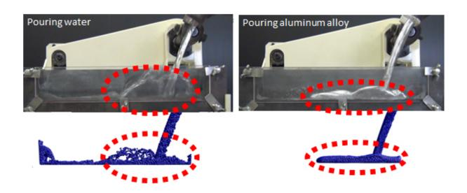
Figure: Trial of the simulation technology in comparison with a pouring experiment with Die Casting shot sleeves: The simulation (below) correctly replicates the differences in motion of water and aluminum alloy, observed in the experiment.
