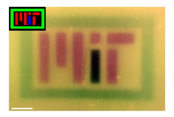
Colored images (insets) were projected onto plates of bacteria containing the RGB system to spell "MIT." The image has been color-corrected in Photoshop to improve contrast. Credit: Felix Moser
