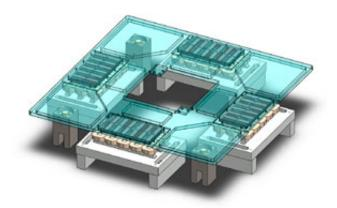
The levitating platform developed by Teo and co-workers contains arrays of permanent magnets floating above several coils of wire. The movement of the platform is controlled by varying the current in the coils. Credit: A\*STAR Singapore Institute of Manufacturing Technology
