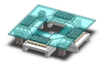
The levitating platform developed by Teo and co-workers contains arrays of permanent magnets floating above several coils of wire. The movement of the platform is controlled by varying the current in the coils. Credit: A\*STAR Singapore Institute of Manufacturing Technology
