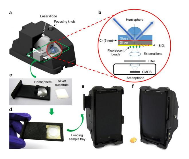
Illustrations and photographs of the mobile phone surface-enhanced fluorescence microscopy device. (a) 3D illustration of the smartphone attachment with the cutaway view of the inner sample stage. (b) Schematic of the Kretschmann configuration implemented in the smartphone attachment. (c,d) Photographs of
