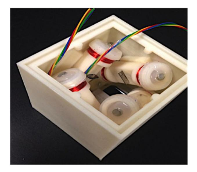
Four sensors arranged in a box measuring about 4 inches on a side make up the test module for the SESE project seismometer. The various sensor orientations allow the instrument to work no matter how it lands on the surface. Credit: Hongyu Yu/ASU
