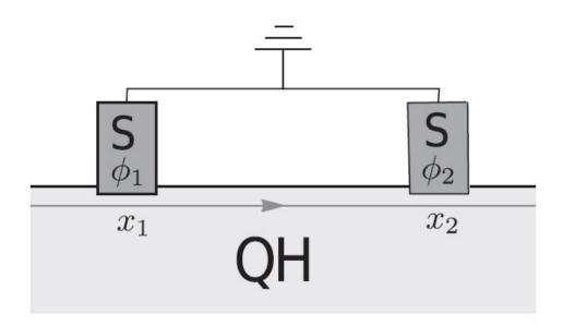
Illustration of the proposed set-up designed to exhibit a superconducting current driven by potential information transfer. Credit: Huang and Nazarov. ©2017 American Physical Society
