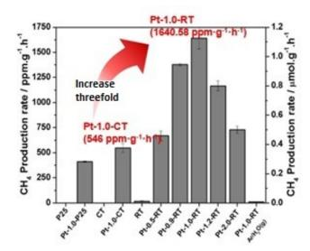
A graph comparing methane production efficiencies between the existing photocatalyst and new photocatalyst developed by the team. Credit: DGIST
