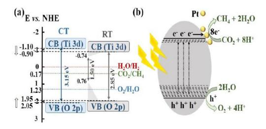
A schematic diagram showing the mechanism of the conversion of carbon dioxide into methane using the reduced titanium dioxide developed by the team. Credit: DGIST
