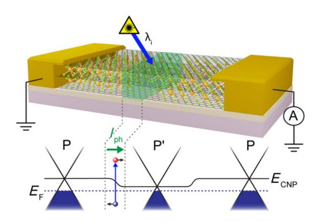
Short-circuit configuration (top) for scanning photocurrent measurements of a p-p'-p junction (p-p' region in green). Schematic band structure (bottom) of each region shows photogenerated carriers drifting under a chemical potential gradient. Credit: *Science Advances* 26 May 2017: Vol. 3, no. 5, e1602617, DOI: 10.1126/sciady.1602617
