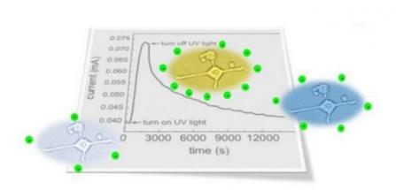
Changes in photocurrent before and after exposure to UV light. Persistent photoconductivity is demonstrated even hours after the UV light has been turned off. This is illustrated by the pictograms showing charge carriers that come into contact with cells at the interface during in vitro experiments. Credit: North Carolina State University
