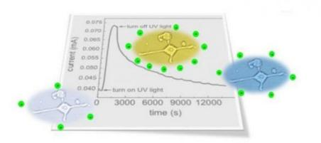
Changes in photocurrent before and after exposure to UV light. Persistent photoconductivity is demonstrated even hours after the UV light has been turned off. This is illustrated by the pictograms showing charge carriers that come into contact with cells at the interface during in vitro experiments. Credit: North Carolina State University
