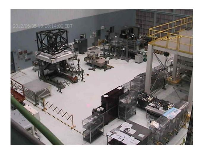
An image taken from one of NASA's two special "Webb-cams," a camera in a giant clean room at NASA Goddard. The Webb-cams focus on what's happening with the very first completed instrument that will fly onboard the James Webb Space Telescope. The flight Integrated Science Instrument Module (ISIM) is at left center. The Ambient Optical Assembly Stand is on the right side of the image. Credit: NASA
