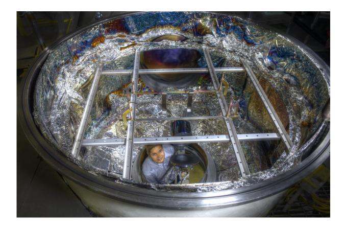
Principal Investigator Manuel Quijada is dwarfed by the two-meter coating chamber where he applies thin films onto telescope mirrors that can be as large as one meter in diameter. The ability to coat large mirrors is key to enabling
