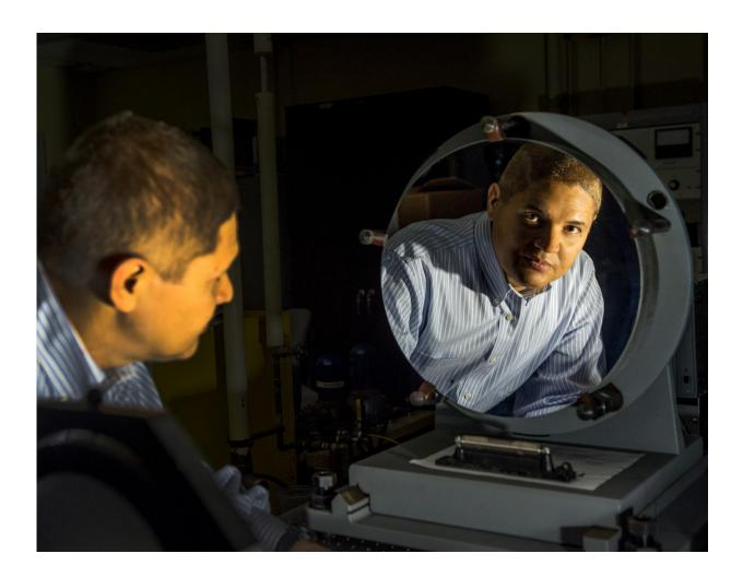
Principal Investigator Manuel Quijada is shown here with the type of optic he and his team would coat with a fluoride film to provide maximum reflectance over a wide spectral range. Credit: NASA/W.Hrybyk
