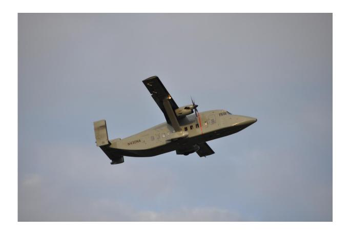
The Wallops Flight Facility Aircraft Office operates the NASA C-23 Sherpa research aircraft available to support airborne science research. The C-23 is a two-engine turboprop aircraft designed to operate under the most arduous conditions, in a wide range of mission configurations. Credit: NASA
