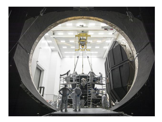
This image, taken from inside the NASA Johnson Space Center Chamber A, captures the James Webb Space Telescope being lifted onto its test stand before sliding it into the chamber. Credit: NASA/Chris Gunn
