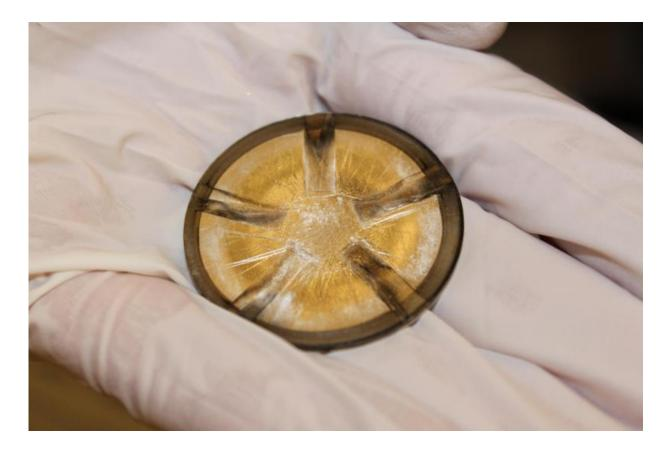
Pure platinum with thin fixed foils of yttrium have been used to create the new nanoalloys that are ten times as effective as pure platinum in fuel cells. Credit: Mia Halleröd Palmgren
