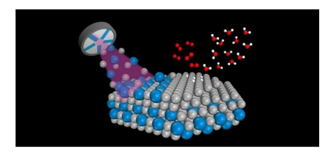
Nanoalloys of platinum (grey) and yttrium (blue) are created using sputtering in a vacuum chamber. This is done by directing plasma (purple) at a piece of platinum with small attached pieces of yttrium. The nanometre-thin alloy films effectively transform oxygen (red) and protons (white) into water. It is this reaction that causes the fuel cell to generate electricity. Credit: Niklas Lindahl
