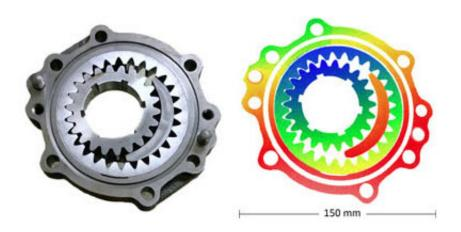
Fig. 8 and 9 show a photograph and measured 3-D image of a 150-mm diameter transmission pump display. Credit: doi:10.1117/1.OE.55.7.074110
