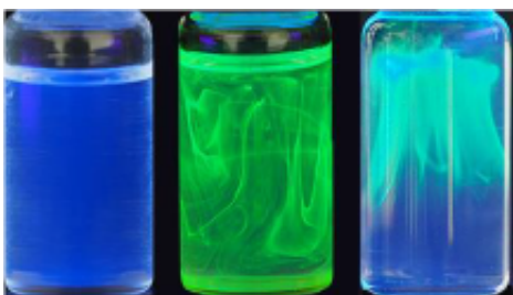
Figure 1: Pictures of LCST system under UV light irradiation at low temperature (left), high temperature (center), and during the course of decreasing temperature (right). Credit: Osaka University
