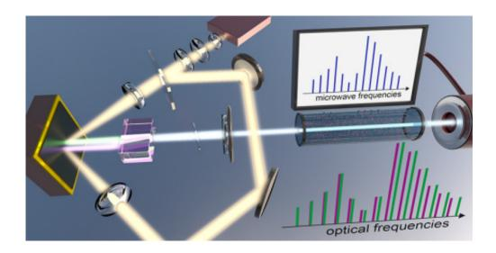
The new method uses a single laser that emits two beams of differing pulse periods. Sending both beams through the sample material creates a beat frequency that can be measured using conventional electronics. Credit: ETH Zurich/Sandro Link
