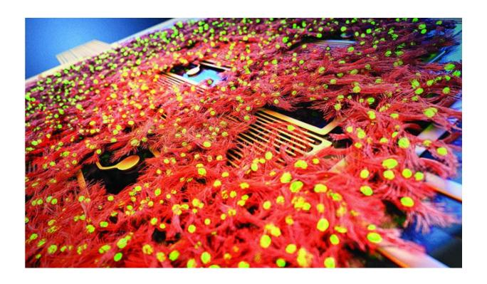
Through "heart-on-a-chip" technology — modeling a human heart on an engineered chip and measuring the effects of compound exposure using microelectrodes — Lawrence Livermore researchers hope to ensure potentially lifesaving new drugs are safe and effective while reducing the need for human and animal testing. Credit: Ryan Chen/LLNL
