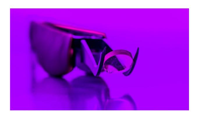
A new 3D printing technique, developed at Lawrence Livermore, could allow scientists to print glass that incorporates different refractive indices in a single flat optic, making finishing cheaper and easier. Credit: Jason Laurea/LLNL
