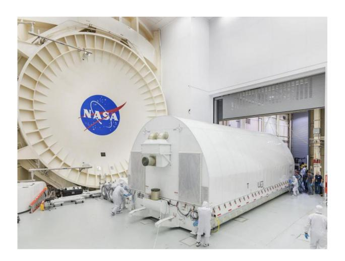
The James Webb Space Telescope is pushed into the clean room of Building 32. Building 32 houses Chamber A, the thermal vacuum chamber where the telescope will have its final thermal vacuum testing. Credit: NASA/Chris Gunn
