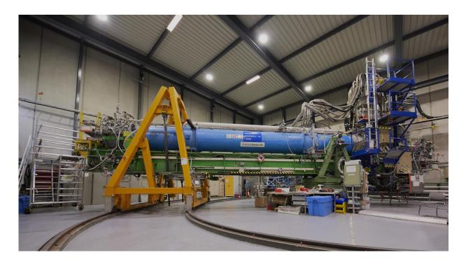
The strong magnet can be found in the blue pipe of the CERN Axion Solar Telescope (CAST) with which researchers seek to capture axions from the sun. Credit: Photo: CERN
