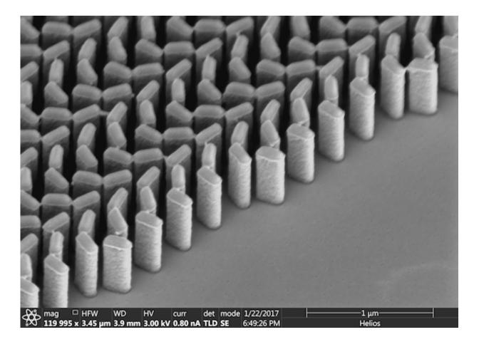
The array of titanium dioxide nanofins can be tailored for any immersion liquid. Credit: Capasso Lab
