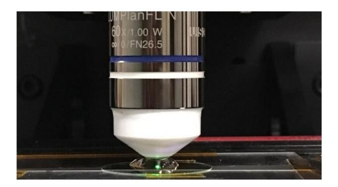
Harvard researchers integrated an immersion meta-lens into a commercial scanning confocal microscope, achieving an imaging spatial resolution of approximately 200 nm. Credit: Capasso Lab/Harvard SEAS
