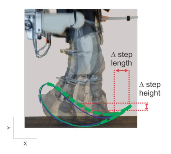
The robotic exosuit delivered forces on the right foot in 19 different directions and angles, interrupting both step length (compromising balance and stability) and step height (compromising stride pattern and energy expenditure). Credit: Cajigas et al., *Sci. Robot.* 2, eaam7749 (2017)
