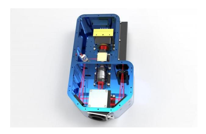
The system can measure centimeter-sized rough objects in fractions of a second with micrometer accuracy - even under disturbances, such as vibrations. Credit: Fraunhofer IPM
