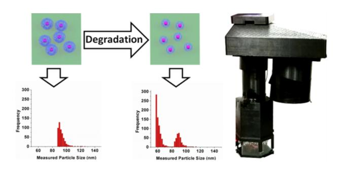
An illustration of a cost-effective method to rapidly monitor the degradation of drug carrying nanoparticles using a chip-scale microscope. Credit: UCLA Ozcan Research Group
