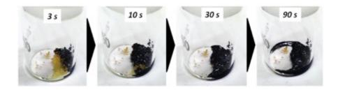
Upon contact of two chemical agent powders at room temperature a viscous dark liquid is formed in a matter of seconds. This is methylammonium polyiodides. Credit: Alexey Tarasov
