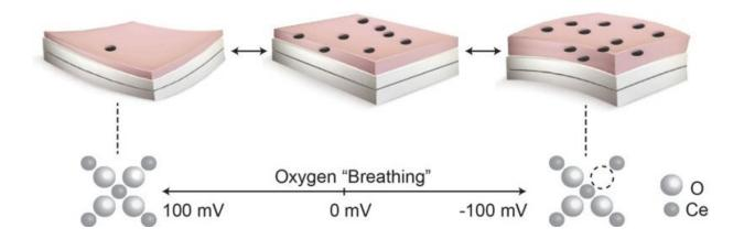
This diagram illustrates how the thin-film material bends from its normal flat state (center) as oxygen is taken up by its structure (right) or released (left). This behavior enables the film's shape to be controlled remotely by changing its electric charge. Credit: Massachusetts Institute of Technology
