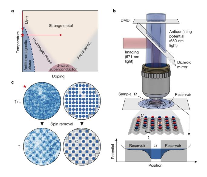
Probing antiferromagnetism in the Hubbard model with a quantum gas microscope. a, Schematic of the two-dimensional Hubbard phase diagram, including predicted phases. b, Experimental set-up. c, Exemplary raw (left) and
