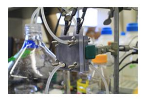
Photograph of the concentration flow cell. Two plates clamp the cell together, which contains two narrow channels fed with either synthetic freshwater or seawater through the plastic lines. Credit: Pennsylvania State University
