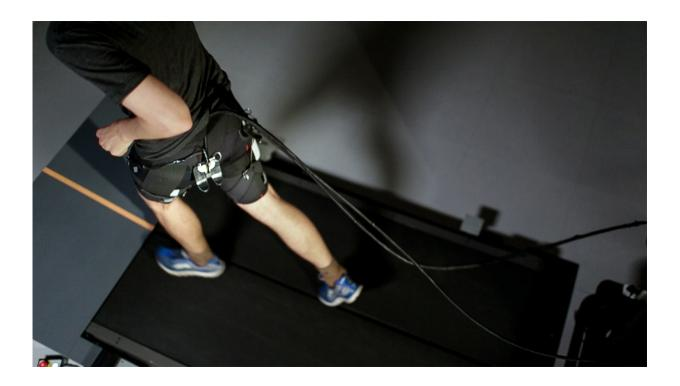
A system of actuation wires attached to the back of the exosuit provides assistive force to the hip joint during running. Credit: The Wyss Institute at Harvard University
