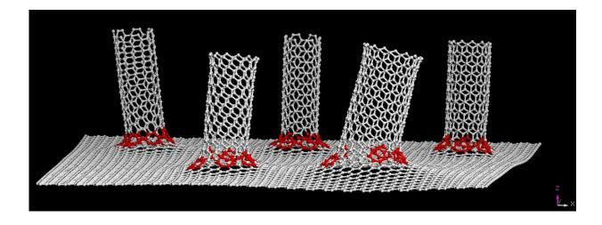
A graphic shows carbon nanotubes covalently bonded to a graphene substrate. The material created at Rice University is being tested as an anode for highcapacity lithium metal batteries. Credit: Tour Group/Rice University
