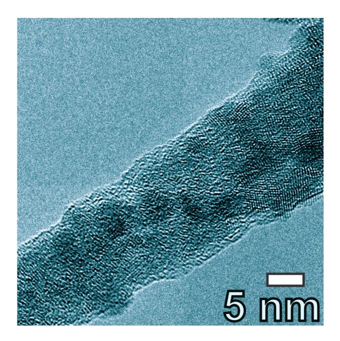
An electron microscope image shows a carbon nanotube evenly coated with lithium metal. Tests on the graphene-carbon nanotube anode created at Rice University show it resists the formation of lithium dendrites that can damage batteries. Credit: Tour Group/Rice University
