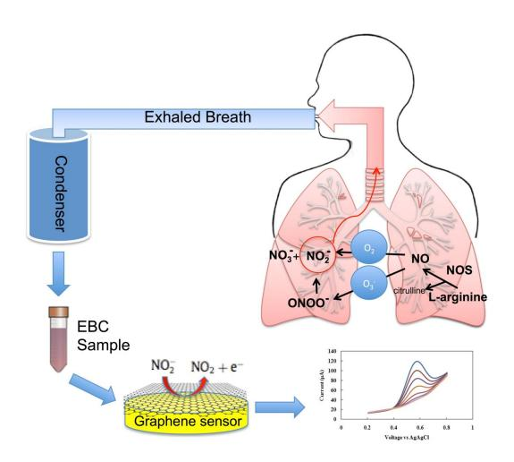
Exhaled breath condensate (tiny droplets of liquid) are rapidly analyzed by a graphene-based nanoelectronic sensor that detects nitrite, a key inflammatory marker in the inner lining of the respiratory airway. Credit: Azam Gholizadeh
