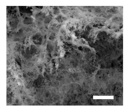
Laser-induced graphene created in the presence of argon gas is superhydrophobic, meaning it avoids water. The process developed at Rice University makes materials that can be superhydrophilic or superhydrophobic from inexpensive materials and in one step. Credit: the Tour Group
