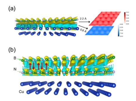
A graphical representation of hexagonal boron nitride (hBN) grown on metal. Credit: U.S. Air Force
