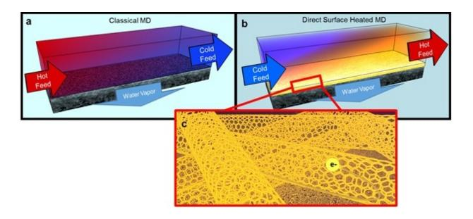
Hot brines used in traditional membrane distillation systems are highly corrosive, making the heat exchangers and other system elements expensive, and limiting water recovery (a). To improve this, UCR researchers developed a self-heating carbon nanotube-based membrane that only heats brine at the membrane surface (b), where the porous carbon nanotube layer acts as a Joule heater (c). Credit: UC Riverside
