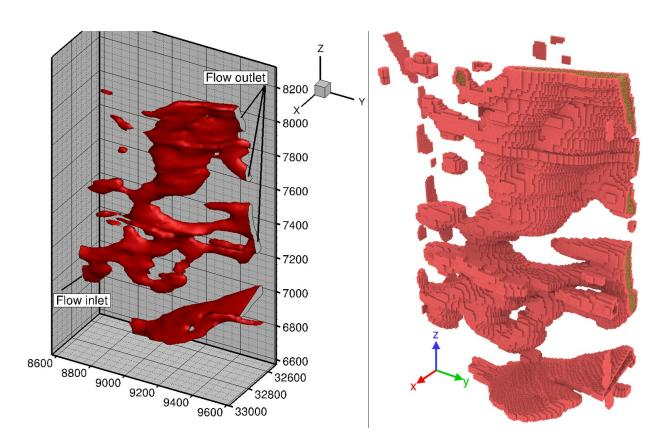
The pore network of the Woodford shale sample (left) and the fluid that fills the pores according to the computer model (right). Credit: Yidong Xia
