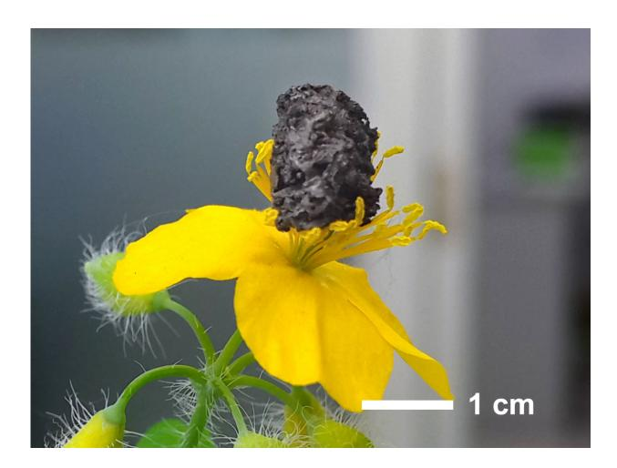
Nanoporous nickel cathodes for lithium oxygen batteries are ultralight, shown here balanced on flower stamens. Credit: American Chemical Society
